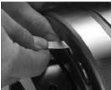
Fig. D-7. Measure RIC before installation.
