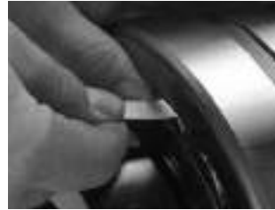
Fig. D-3. Measure RIC before installation.
